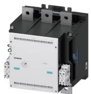
vacuum contactor AC-3e 630 A, 335 kW / 400 V, AC-3 820 A, 450 kW / 400 V, Ue 690 V, 3-pole, Uc: 200-240 V AC(50/60 Hz) drive: conventional auxiliary contacts 4 NO + 4 NC main circuit: busbar control and auxiliary circuit: screw terminal
