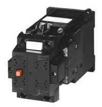
Contactor, Size 2, 2-pole, DC-3 and 5, 32 A Auxiliary contacts 22 (2 NO + 2 NC) 24V DC DC operation Operating range 0.85-1.1 UN
