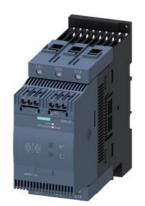
SIRIUS soft starter S3 106 A, 55 kW/400 V, 40  $^{\circ}\text{C}$  200-480 V AC, 24 V AC/DC Screw terminals
