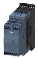
SIRIUS soft starter S2 72 A, 37 kW/400 V, 40 °C 200-480 V AC, 110-230 V AC/DC Screw terminals
