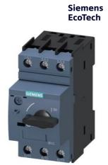
Circuit breaker size S0 for transformer protection A-release 18...25 A N-release 400 A screw terminal Standard switching capacity
