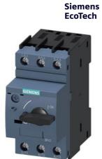
Circuit breaker size S0 for transformer protection A-release 13...20 A N-release 325 A Screw terminal Standard switching capacity
