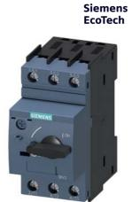
Circuit breaker size S00 for transformer protection A-release 0.7...1 A N-release 21 A screw terminal Standard switching capacity
