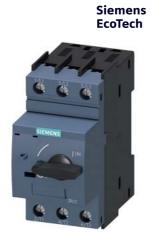
Circuit breaker size S00 for starter combination Rated current 4 A N release 52 A screw terminal Standard switching capacity
