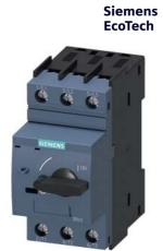
Circuit breaker size S00 for starter combination Rated current 0.5 A N-release 6.5 A screw terminal Standard switching capacity
