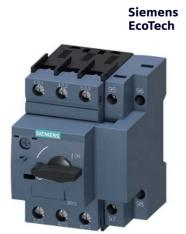
Circuit breaker size S0 for motor protection, CLASS 10 with overload relay function A-release 23...28 A N-release 364 A screw terminal Standard switching capacity
