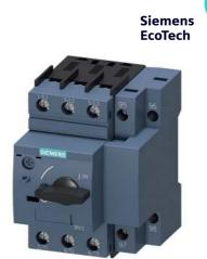
Circuit breaker size S00 for motor protection, CLASS 10 with overload relay function A-release 1.4...2 A N-release 26 A screw terminal Standard switching capacity
