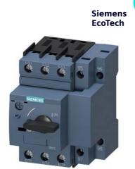
Circuit breaker size S00 for motor protection, CLASS 10 with overload relay function A-release 0.18...0.25 A N-release 3.3 A screw terminal Standard switching capacity
