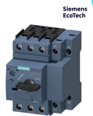
Circuit breaker size S00 for motor protection, CLASS 10 with overload relay function A-release 0.11...0.16 A N-release 2.1 A screw terminal Standard switching capacity
