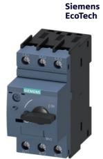
Circuit breaker size S0 for motor protection, CLASS 10 A-release 18...25 A N-release 325 A Screw terminal Standard switching capacity
