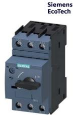
Circuit breaker size S00 for motor protection, CLASS 10 A-release 10...16 A N-release 208 A screw terminal Standard switching capacity
