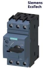
Circuit breaker size S00 for motor protection, CLASS 10 A-release 0.18...0.25 A N-release 3.3 A screw terminal Standard switching capacity
