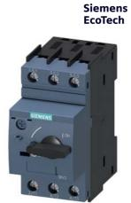
Circuit breaker size S00 for motor protection, CLASS 10 A-release 0.14...0.2 A N-release 2.6 A screw terminal Standard switching capacity
