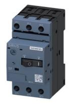
Circuit breaker size S00 for motor protection, CLASS 10 A-release 9...12 A N-release 156 A Screw terminal Standard switching capacity
