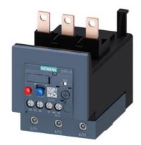
Overload relay 80...100 A Thermal For motor protection Size S3, Class 10 Contactor mounting Main circuit: Screw Auxiliary circuit: Screw Manual-Automatic-Reset
