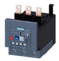
Overload relay 28...40 A Thermal For motor protection Size S3, Class 10 Contactor mounting Main circuit: Screw Auxiliary circuit: Screw Manual-Automatic-Reset
