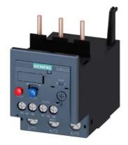
Overload relay 36...45 A Thermal For motor protection Size S2, Class 10 Contactor mounting Main circuit: Screw Auxiliary circuit: Screw Manual-Automatic-Reset
