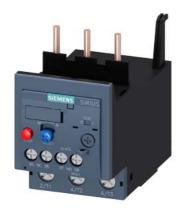
Overload relay 28...40 A Thermal For motor protection Size S2, Class 10 Contactor mounting Main circuit: Screw Auxiliary circuit: Screw Manual-Automatic-Reset
