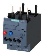
Overload relay 9.0...12.5 A Thermal For motor protection Size S0, Class 10 Contactor mounting Main circuit: Screw Auxiliary circuit: Screw Manual-Automatic-Reset
