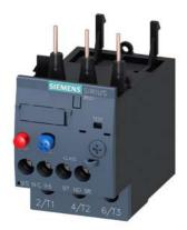
Overload relay 2.8...4.0 A Thermal For motor protection Size S0, Class 10 Contactor mounting Main circuit: Screw Auxiliary circuit: Screw Manual-Automatic-Reset
