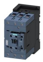
power contactor, AC-3e/AC-3, 110 A, 55 kW / 400 V, 3-pole, 24 V AC, 50/60 Hz, auxiliary contacts: 1 NO + 1 NC, screw terminal, size: S3  $\,$
