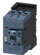
power contactor, AC-3e/AC-3, 95 A, 45 kW / 400 V, 3-pole, 20-33 V AC/DC, 50/60 Hz, with integrated varistor, auxiliary contacts: 1 NO + 1 NC, screw terminal, size: S3
