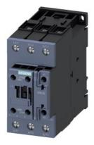
power contactor, AC-3e/AC-3, 80 A, 37 kW / 400 V, 3-pole, 175-280 V AC/DC, 50/60 Hz, with integrated varistor, auxiliary contacts: 1 NO + 1 NC, screw terminal, size: S2
