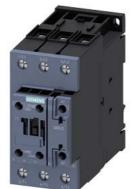
power contactor, AC-3e/AC-3, 80 A, 37 kW / 400 V, 3-pole, 110 V AC, 50/60 Hz, auxiliary contacts: 1 NO + 1 NC, screw terminal, size: S2  $\,$
