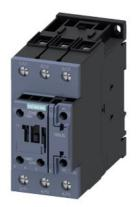
power contactor, AC-3e/AC-3, 65 A, 30 kW / 400 V, 3-pole, 175-280 V AC/DC, 50/60 Hz, with integrated varistor, auxiliary contacts: 1 NO + 1 NC, screw terminal, size: S2
