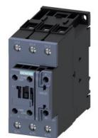
power contactor, AC-3e/AC-3, 65 A, 30 kW / 400 V, 3-pole, 83-155 V AC/DC, 50/60 Hz, with integrated varistor, auxiliary contacts: 1 NO + 1 NC, screw terminal, size: S2
