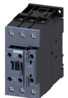
power contactor, AC-3e/AC-3, 51 A, 22 kW / 400 V, 3-pole, 110 V AC, 50/60 Hz, auxiliary contacts: 1 NO + 1 NC, screw terminal, size: S2
