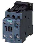
power contactor, AC-3e/AC-3, 32 A, 15 kW / 400 V, 3-pole, 110 V DC, auxiliary contacts: 1 NO + 1 NC, screw terminal, size: S0
