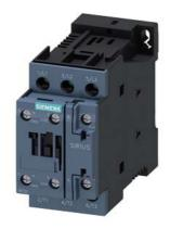
power contactor, AC-3e/AC-3, 25 A, 11 kW / 400 V, 3-pole, 110 V DC, auxiliary contacts: 1 NO + 1 NC, screw terminal, size: S0  $\,$
