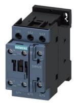
power contactor, AC-3e/AC-3, 17 A, 7.5 kW / 400 V, 3-pole, 110 V AC, 50/60 Hz, auxiliary contacts: 1 NO + 1 NC, screw terminal, size: S0
