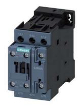
power contactor, AC-3e/AC-3, 12 A, 5.5 kW / 400 V, 3-pole, 220 V DC, auxiliary contacts: 1 NO + 1 NC, screw terminal, size: S0  $\,$
