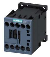
power contactor, AC-3e/AC-3, 16 A, 7.5 kW / 400 V, 3-pole, 24 V DC, auxiliary contacts: 1 NC, screw terminal, size: S00  $\,$
