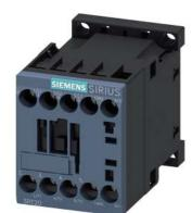
power contactor, AC-3e/AC-3, 12 A, 5.5 kW / 400 V, 3-pole, 220 V DC, auxiliary contacts: 1 NO, screw terminal, size: S00
