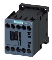
power contactor, AC-3e/AC-3, 9 A, 4 kW / 400 V, 3-pole, 110 V AC, 50/60 Hz, auxiliary contacts: 1 NO, screw terminal, size: S00  $\,$
