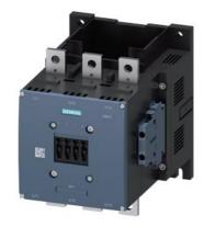
power contactor, AC-3e/AC-3 500 A, 250 kW / 400 V without operating mechanism 3-pole, auxiliary contacts 2 NO + 2 NC main circuit: busbar control and auxiliary circuit: screw terminal
