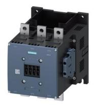
power contactor, AC-3e/AC-3 400 A, 200 kW / 400 V without operating mechanism 3-pole, auxiliary contacts 2 NO + 2 NC main circuit: busbar control and auxiliary circuit: screw terminal
