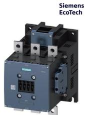
power contactor, AC-3e/AC-3 265 A, 132 kW / 400 V AC (50-60 Hz) / DC Uc: 220-240 V 3-pole, auxiliary contacts 2 NO + 2 NC drive: conventional main circuit: busbar control and auxiliary circuit: screw terminal
