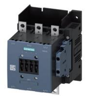
power contactor, AC-3e/AC-3 150 A, 75 kW / 400 V without operating mechanism 3-pole, auxiliary contacts 2 NO + 2 NC without operating mechanism main circuit: busbar control and auxiliary circuit: screw terminal
