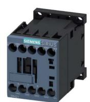
Coupling contactor relay, 3 NO+1 NC 24 V DC, 0.85-1.85\*US with integrated suppressor diode Size S00 screw terminal
