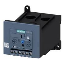
Overload relay 32...115 A Electronic For motor protection Size S3, Class 5E...30E Stand-alone installation Main circuit: Straight-through transformer Auxiliary circuit: Screw Manual-Automatic-Reset
