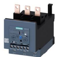
Overload relay 32...115 A Electronic For motor protection Size S3, Class 5E...30E Contactor mounting Main circuit: Screw Auxiliary circuit: Screw Manual-Automatic-Reset
