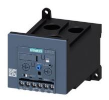
Overload relay 12.5...50 A Electronic For motor protection Size S3, Class 5E...30E Stand-alone installation Main circuit: Straight-through transformer Auxiliary circuit: Screw Manual-Automatic-Reset
