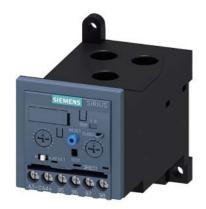
Overload relay 12.5...50 A Electronic For motor protection Size S2, Class 5E...30E Stand-alone installation Main circuit: Straight-through transformer Auxiliary circuit: Screw Manual-Automatic-Reset Internal ground fault detection
