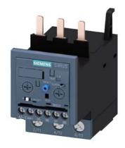
Overload relay 12.5...50 A Electronic For motor protection Size S2, Class 5E...30E Contactor mounting Main circuit: Screw Auxiliary circuit: Screw Manual-Automatic-Reset Internal ground fault detection
