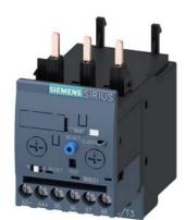
Overload relay 3...12 A Electronic For motor protection Size S0, Class 5...30 Contactor mounting Main circuit: Screw Auxiliary circuit: Screw Manual-Automatic-Reset Internal ground fault detection
