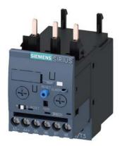
Overload relay 0.1...0.4 A Electronic For motor protection Size S0, Class 5...30 Contactor mounting Main circuit: Screw Auxiliary circuit: Screw Manual-Automatic-Reset Internal ground fault detection
